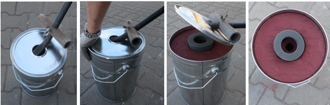
Figure 2: opening the charged single use crucible I with a crucible opener
